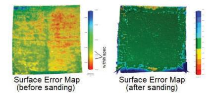
The radio frequency (RF) subsystem team is completing resurfacing of the reflector at the LaRC test range used for High Gain Antenna (HGA) testing. The images show the before and after surface measurements, illustrating the effectiveness of the "prime and sand process."
