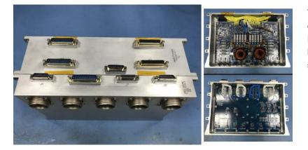
The Power subsystem team has completed testing of the Array Battery Interface Slice (ABIS) breadboard, showing good power sharing across the three regulators
