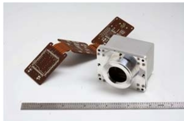
Figure B.2.5-8. Ample radiation shielding encloses a miniature focal plane assembly for a STAR1000 CMOS APS.
