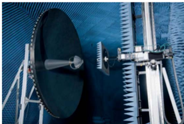
Figure B.2.7-29. Juno's 3-m HGA (X/Ka-band) provides the basis for the Europa HGA.
