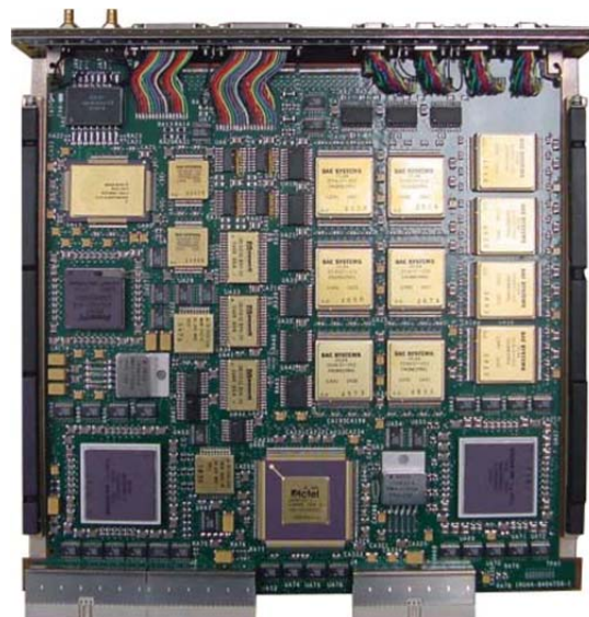
Figure B.2.7-37. The RAD750 provides high heritage for both the C&DH electronics and FSW designs.
