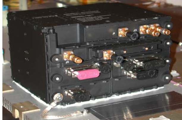
Figure C.2.4-29. The SDST product line provides the mission-critical communications link to Earth.
