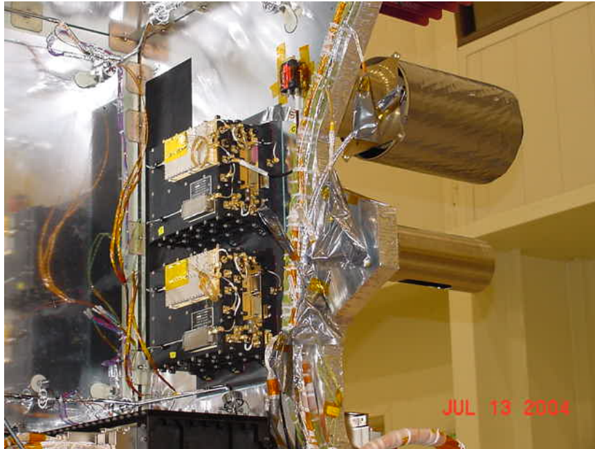
Figure D.2.4-22. The Electra Payload, as shown on MRO, provides the basis for UST Relay Communications for the Europa Lander..
