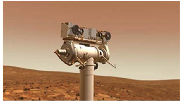
Figure D.2.2-8. The MER Pancam mounted on a two-axis-gimballed platform atop a 1.5-m-tall mast provides a good analog for the Europa Lander SIS.
