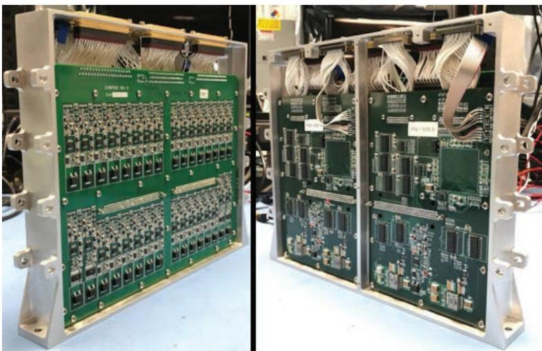
The Power subsystem team has completed the build and is proceeding with bench top testing of the Power Switch Slice assembly.
