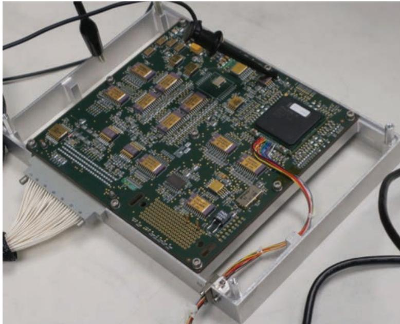
The Propulsion Module Electronics (PME) team has completed the build of the Mezzanine card for the PME, shown in initial bench top testing.
